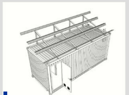
Phase 3: Installation of metallic frame for panels.
